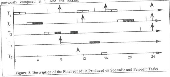
all periodic requests with deadline 14 be completed since 14 is the earliest deadline followed by an idle time in the EDL schedule. At time 13, the system laxity gets higher enough so as to execute the critical section S<sup>2</sup> non-preemptively. T<sub>1</sub> finally completes at time 15. Task T<sub>2</sub> which arrived at time 11 is executed between times 15 and 16. The effective schedule produced within the hyperperiod is described in Figure 3.
