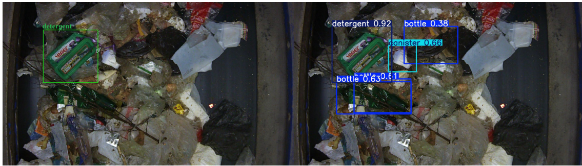
Figure 5. Comparison between labels (left) and predictions (right) for the baseline model
