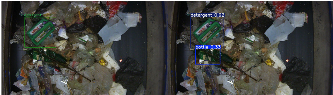
Figure 7. Comparison between labels (left) and predictions (right) for the model trained with 2,500 more synthetic images
