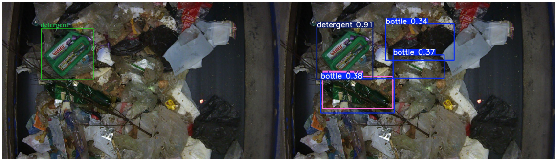
Figure 9. Comparison between labels (left) and predictions (right) for the model trained with 5000 more synthetic images
