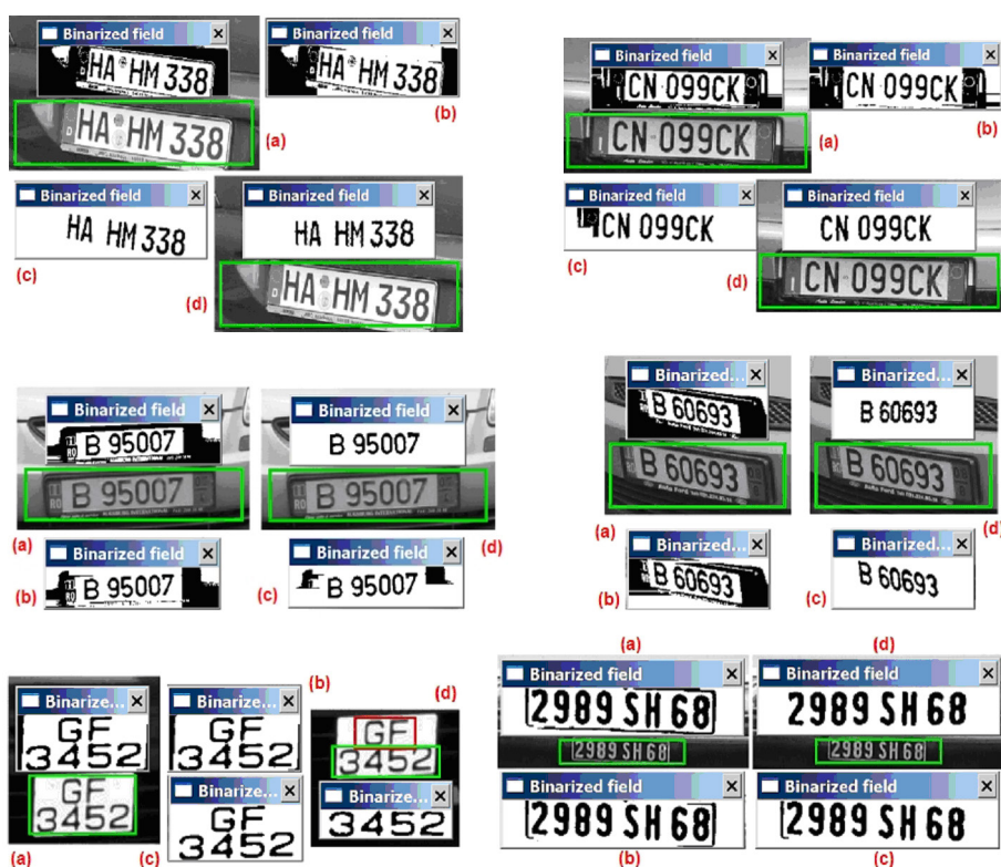
Figure 4. Segmentation stages outcomes after: (a) ROI binarization; (b) filtering long horizontal lines; (c) filtering#1; (d) eliminating possible rotation, slant and/or tilt, and filtering#2
