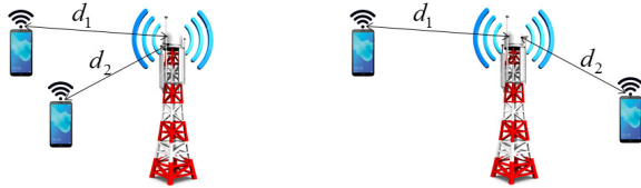
Figure 4. By the fixed distances from two transmitters to the base station, model (1) — (4) gives anyway the same signal-to-interference ratio for each transmitter, and the utilities are constant
