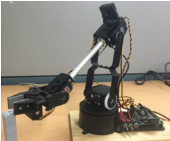
Figure 3. Camera mounted on the shoulder of the robot arm
