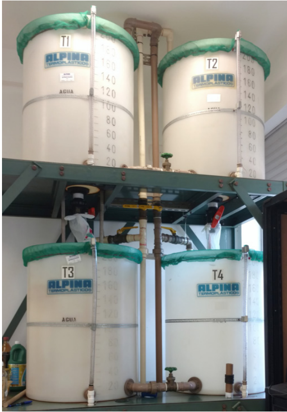
Figure 5. Four tanks interactive system
