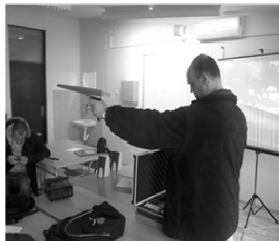
Figure 4. The positions of measuring points in the cabinet M8 and the measurement procedure with the instrument SPECTRAN HF 60105
