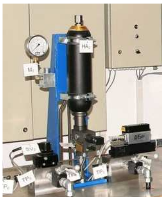
Figure 22. Dynamic test bench for pilot stages
