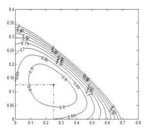
**Figure 2.** Contour levels of the Lagrangian function  $L_{h,1,4}(x,\eta^*)$  of the equivalent model.
