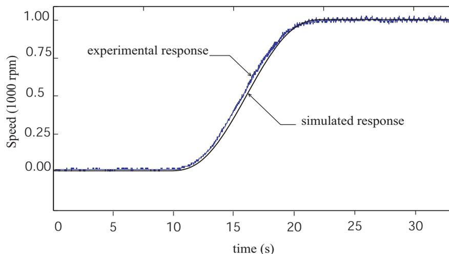
**Figure 15.** Comparison of Experimental and Simulated Responses
