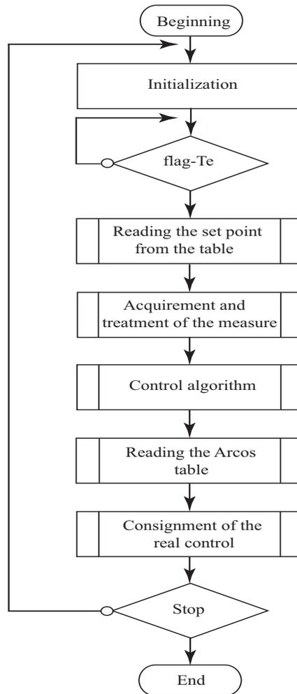
Figure 10. Flow Chart of the Control algorithm
