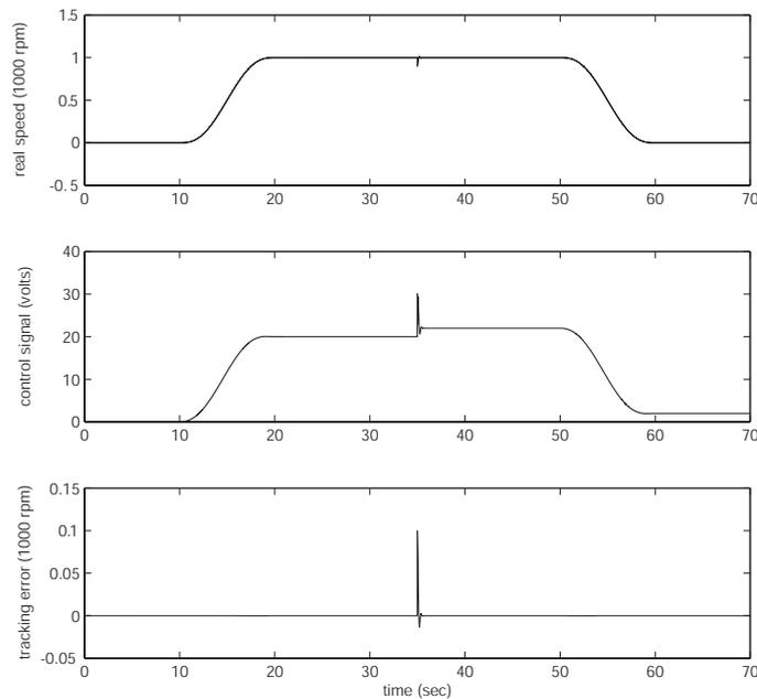
**Figure 6.** Simulation results in the case of flatness-based RST polynomial controller. Variation with 50% of the  $a_i$  parameters model
