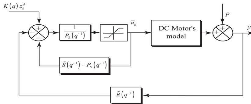
**Figure 1.** Flatness-based RST Polynomial Controller for DC Motor Model
