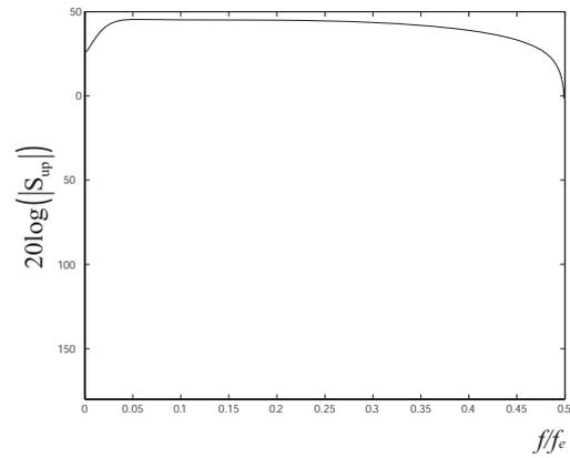
**Figure 4.** Input sensitivity function: case of high frequency noises elimination
