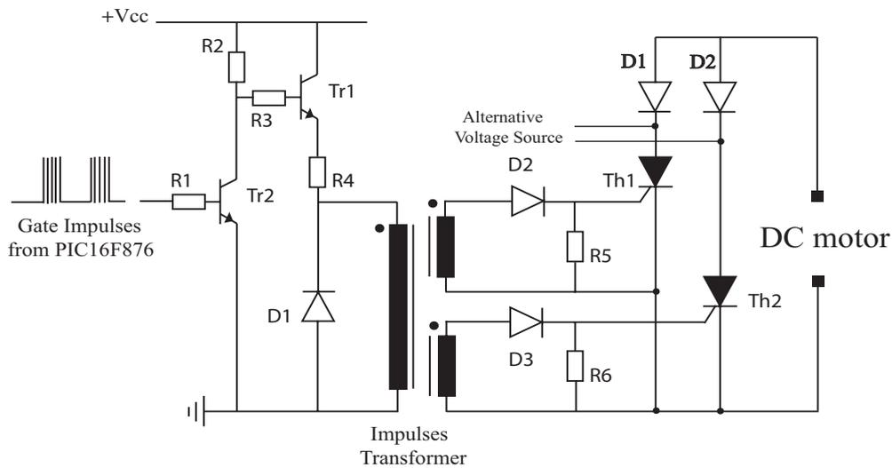
**Figure 8.** AC-DC Power Converter Control
