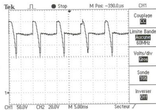
**Figure 14.** Control Voltage of DC Motor
