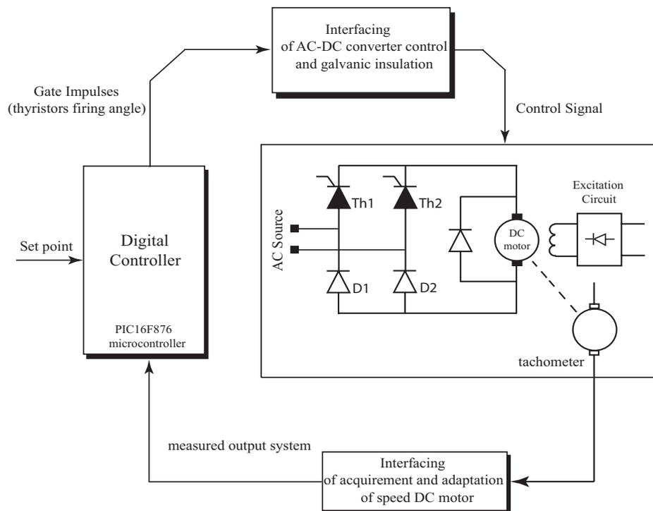
**Figure 7.** Hardware Architecture of the Digital Control System
