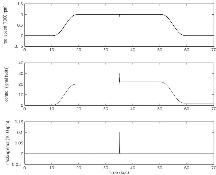
**Figure 5.** Simulation results in the case of flatness-based RST polynomial controller
