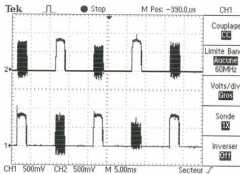
**Figure 13.** State of Thyristors Conduction
