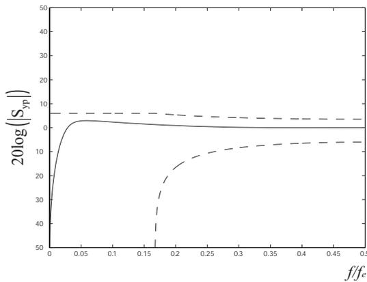
**Figure 3.** Output sensitivity function: case of static disturbance rejection
