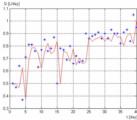
**Figure 10.** Testing results of neural model of AD with input  $S_{I0}$  output  $Q$ , trained with generated data (\* real data; – neural model)
