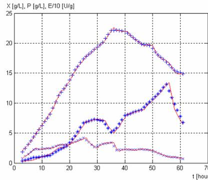
**Figure 3.** Testing results of neural models for batch SOD production including unregulated DO (real data for  $^+X$ ,  $^+P$ ,  $^+E/10$ ; – neural models)
