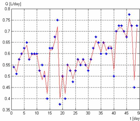
**Figure 11.** Testing results of neural model of AD with input  $S_{I0}$  output  $Q$ , trained with real experimental data (\* real data; – neural model)
