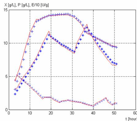
**Figure 4.** Testing results of neural models for batch SOD production including regulated DO (real data for  $^+X$ ,  $^+P$ ,  $^+E/10$ ; – neural models)
