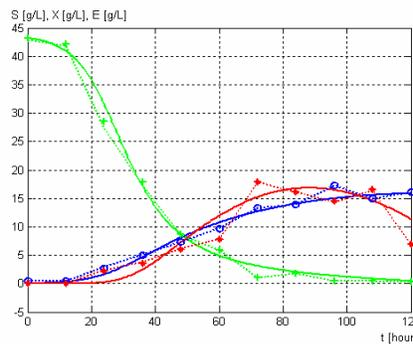
**Figure 1.** Testing results for deterministic and neural model for batch SOD production (real data for \*S, °X, \*E; – deterministic model; neural model)
