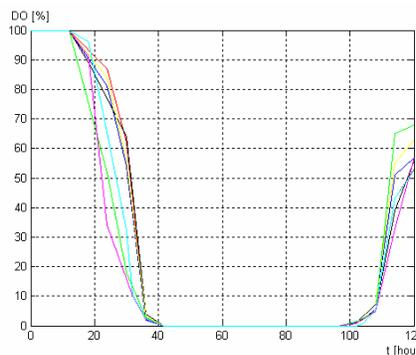
**Figure 2.** Inputs of neural models of batch process for SOD production including unregulated DO
