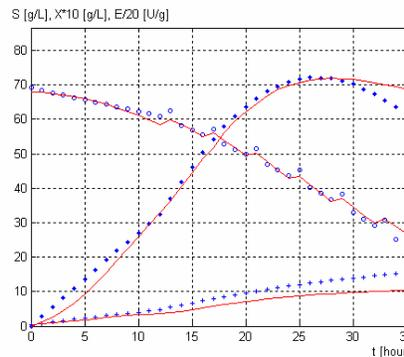
**Figure 9.** Testing results of hybrid model for fed-batch SOD production (filtered data for °S, +X.10, \*E/20; – hybrid model)
