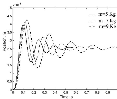
**Figure 2.** One step position evolutions of the LTSRSM for various plunger weight values
