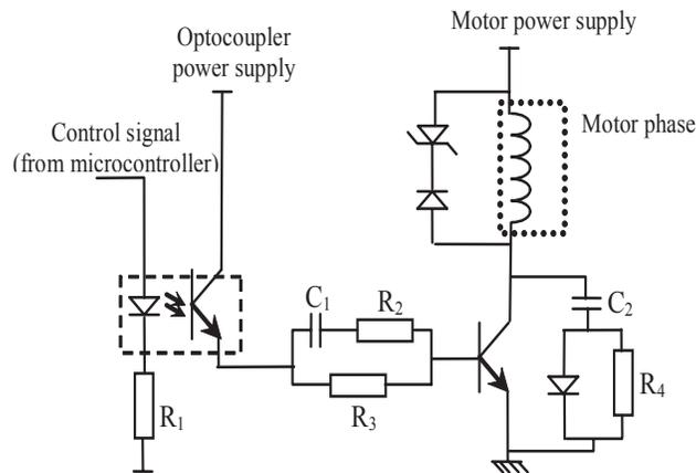
**Figure 9.** Structure of one converter leg
