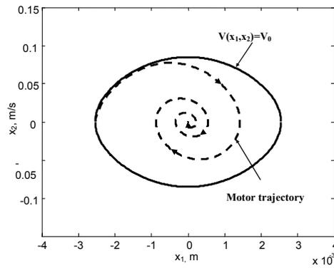
**Figure 5.** Simulated motor trajectory and stable boundary
