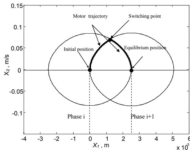
**Figure 7.** Definition of the switching point of the bang-bang control
