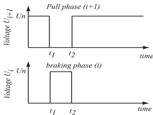
**Figure 4.** Sequence of the control voltages of the bang-bang control
