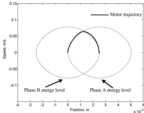
**Figure 9.** Simulated motor trajectory by application of the bang-bang control
