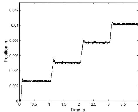
**Figure 12.** Four steps position evolution by application of the bang-bang control
