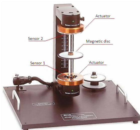
Figure 1. Magnetic Levitation System made by ECP (ECP, 1999).
