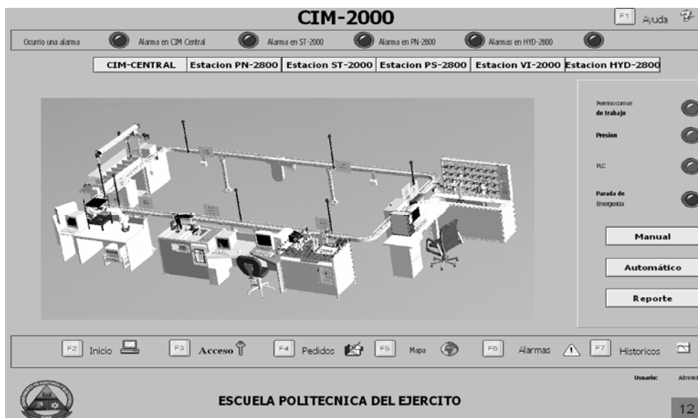
Figure 1. Second HMI CIM 2000 prototype using the GEDIS guideline. In this screen the user has a clear situation awareness (alarm information at the top) and a good access to alarms window or levels of automation (manual control, automatic control)
