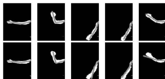
Figure 12. Visual comparison for the same frames of limb tracking using automatic parameter selection and without. Top row using the parameters obtained with the designed algorithm. Bottom row using a set of predefined parameters. As we can observe in the top row we obtain a better adjustment.
