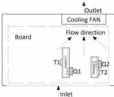
**Figure 4.** Experimental setup Q<sub>1</sub> and Q<sub>2</sub> - MOSFETs, T<sub>1</sub>, T<sub>2</sub> - Sensors
