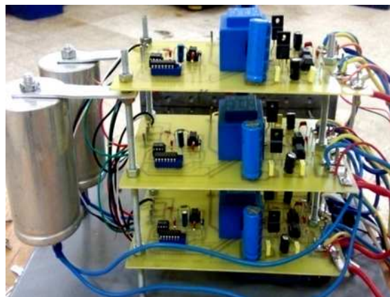
Control card and capacitors
