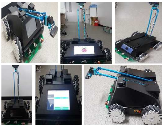
Figure 9. Intelligent Surveillance Robot SMART-I
