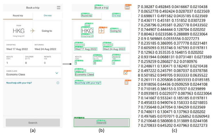
Figure 12. Result of GUI element detection: (a) original GUI; (b) detection result; (c) result details
